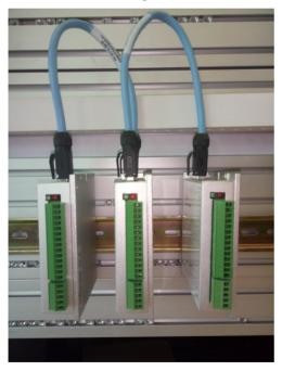
We don't need to setup address for connecting expansion modules. The real address in the net depend on the turn that KincoBuilder configurate hardware.
